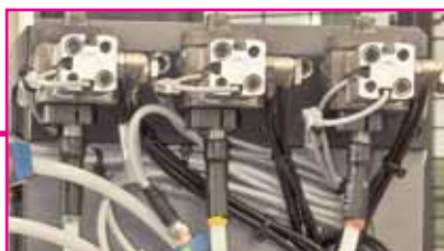
Solid punch rivet docking, here for 3 rivet lengths
