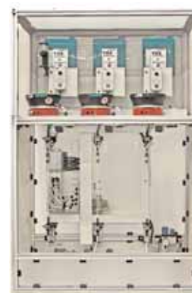
Several separators in the rivet supply module, here for 7 rivet lengths
