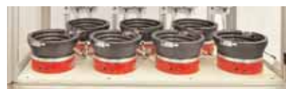
Several separators in the rivet supply module, here for 7 rivet lengths
