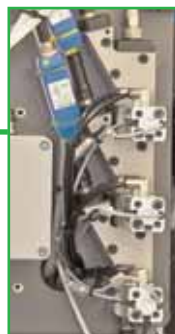
Solid punch rivet docking, here for 3 rivet lengths
